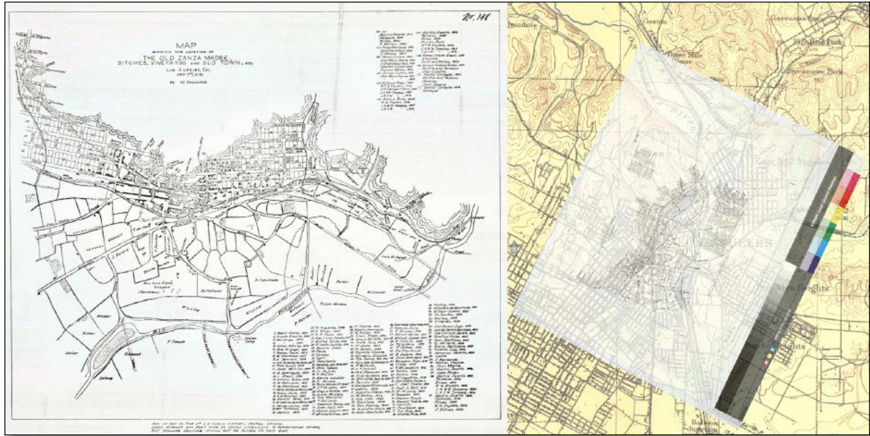
Figure 4-5. Example of georeferencing for M. Kelleher's 1875 "Map showing the locations of the Old Zanja Madre, Ditches, Vineyards and Old Town, etc." At left, original image: Rio Porciúncula (Los Angeles River) crosses the page from left to right, with a river island at lower left and extensive tracts of willows along the river; irrigation ditches, gardens and vineyards lie between the river and the streets and buildings of the old town, built next to the mountains shown by contour lines across the top of the map. At right, the georeferenced map is semi-transparent to show its new spatial alignment with an 1894 USGS topo map; the Los Angeles River flows southward from the top left to the bottom of the map.
